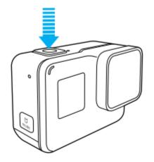
The camera powers on, beeps several times, and automatically begins capturing video. The camera status lights blink while the camera is recording.
